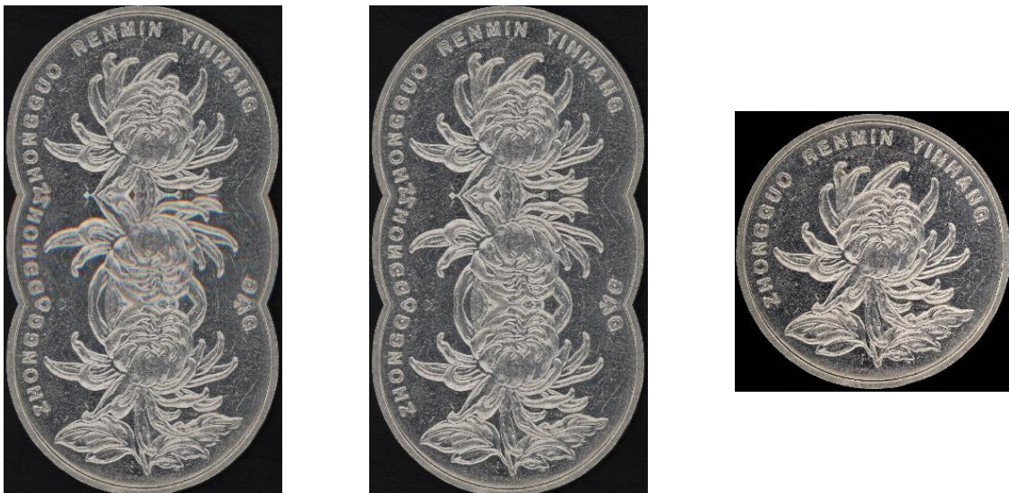
Figure 4: Concept sketch of the backward motion rejection. All images were taken with the same movement pattern of the linear stage which includes a backward drive. The left image uses no direction information, the middle one corrects the color plane shift and the right one suppresses all repeated image content.
