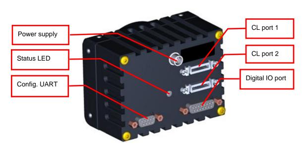
Figure 16: The allPIXA wave camera connections and status LED
