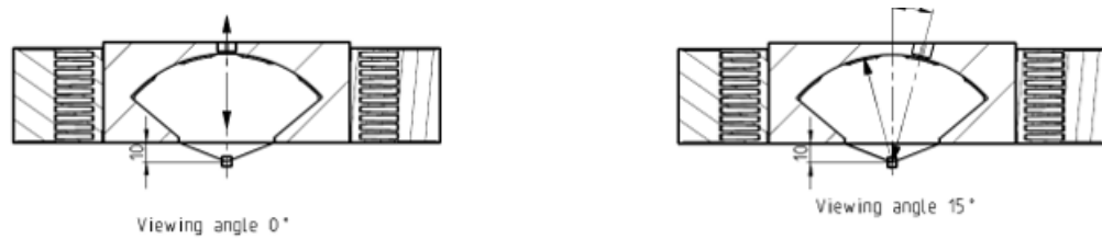
Figure 5-15 Different viewing angles for Tube light version
