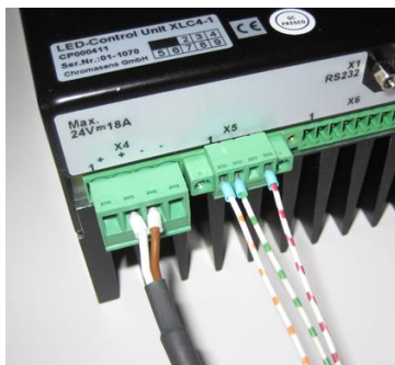
Figure 8-2: Connecting the fan to the XLC4 with fan monitoring
