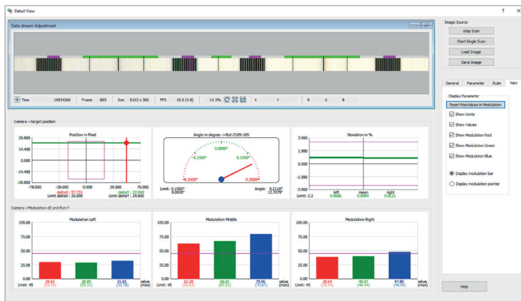
Figure 3.1: GEN<i>CAM supported GCT Software: Camera alignment target and real time measurement of camera position, MTF and resolution.
