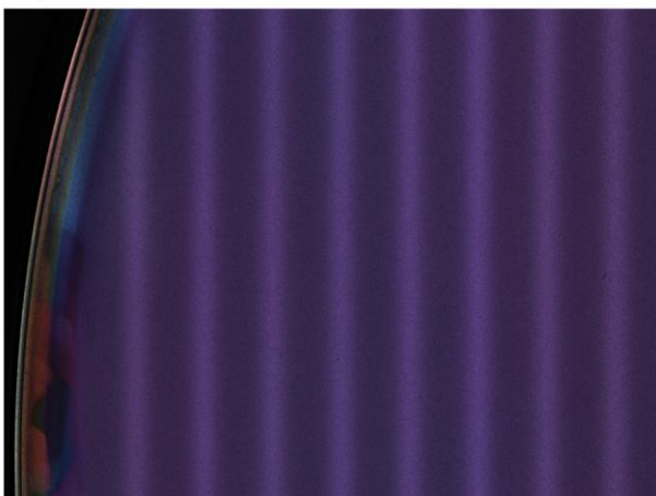
Unprocessed wafer without diffuser in coax-brightfield
